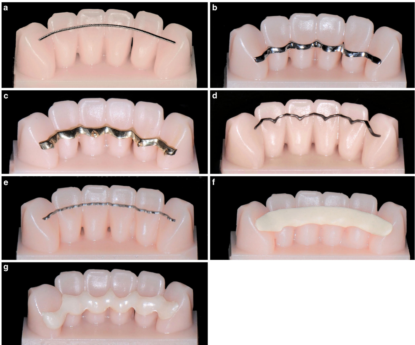
Fig. 2 Tested retainers—conventional twistflex retainers ( a ) and six commercially available computer-aided design/computer-aided manufacturing (CAD/CAM) retainers ( b–f ) were tested. The CAD/CAM retainers were made from cobalt–chromium ( b ), gold ( c ), titanium grade 5 ( d ), nickel–titanium ( e ), polyetheretherketone ( f ) and zirconia ( g )
