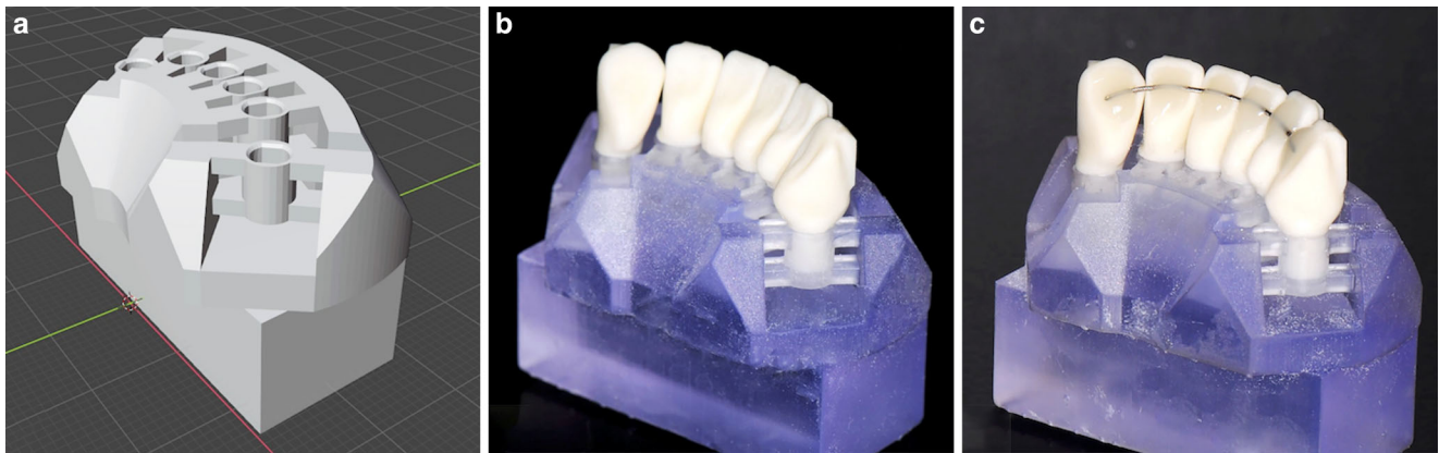
Fig. 1 In vitro tooth model. The model base and the teeth were planned and manufactured using computer-aided design/computer-aided manufacturing (CAD/CAM) technology. The model base contained flexible bars that simulated physiological tooth mobility (a). All teeth provided planar loading sites on the vestibular surface and were embedded in the model base (b). Retainers were bonded on the models (c)
